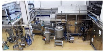
Butter-production lines made by B e H o spol. s r.o. are controlled on a high level of automation; they are fully automatic in various modes such as washing and sanitation. The central control system provides all important information about the production process and butter parameters.
